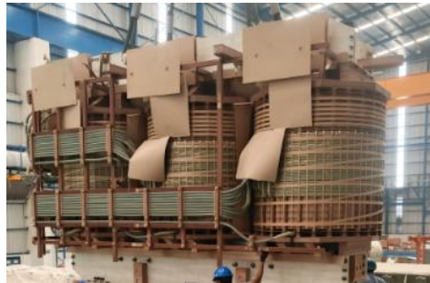
Gambar 2. 4 Belitan Transformator (Winding)
