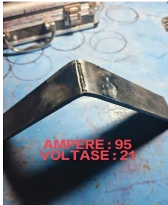
Gambar 4. 2 Hasil Uji Bending U-Channel 1
