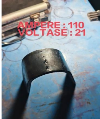
Gambar 4. 3 Hasil Uji Bending U-Channel 2
