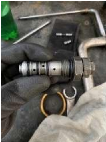
Gambar 4. 9 Spool LS Valve Sudah di Reseal
