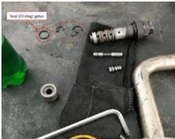
Gambar 4. 8 Kerusakan Seal LS Spool Valve
