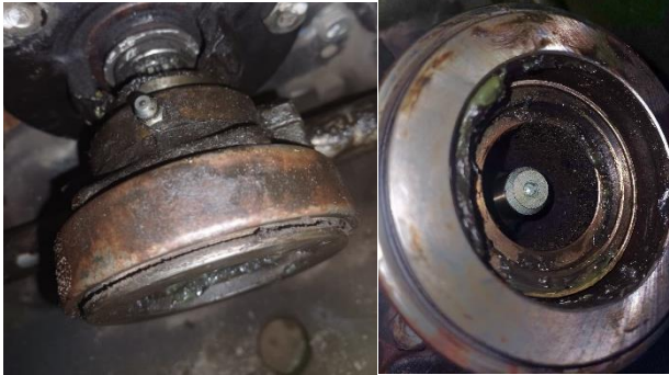
Gambar 4. 4 Pemeriksaan Release Bearing
