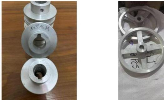
Gambar 4. 6 *Driver pulley 3 inch & driven pulley 8 inch*
