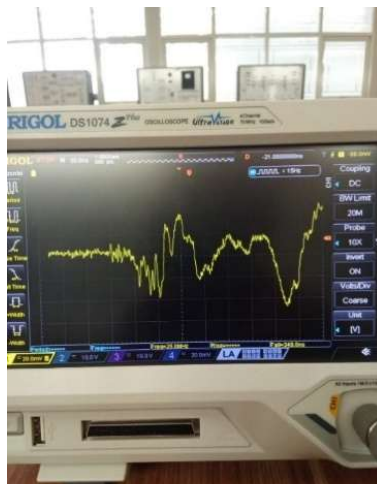
Gambar 4. 2 Pengujian Sensor Pir (LOW)
