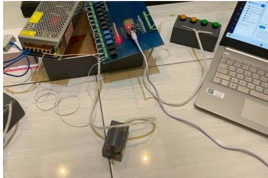
Gambar 4.2 Kerja tombol start dan tombol stop terhadap penegndalian motor Dc
